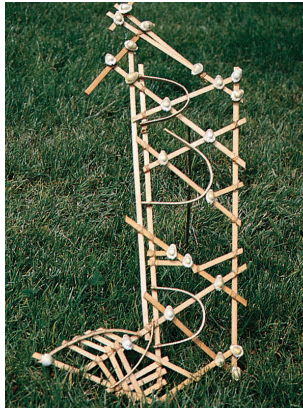
Figure P.3 A navigational chart ( rebillib ) of the Marshall Islands. Sticks represent a series of regular wave patterns (swells). Curved sticks show waves bent by the shorelines of individual islands. Islands are represented by shells.
